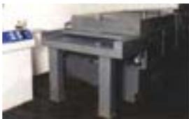
Our Etching machine is probably the largest in the nameplate industry it can Etch a sheet at 2400 x 1200 mm ( 8ft x 4ft ) Maximum Width is 48 " ( 1220 mm ) but the length is not really restricted.
